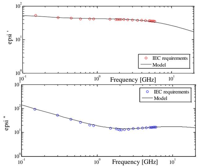
Fig. 2.  $\epsilon'$  and  $\epsilon''$  as functions of frequency: analytical model fit with IEC 62209-2 dielectric requirements [5]
