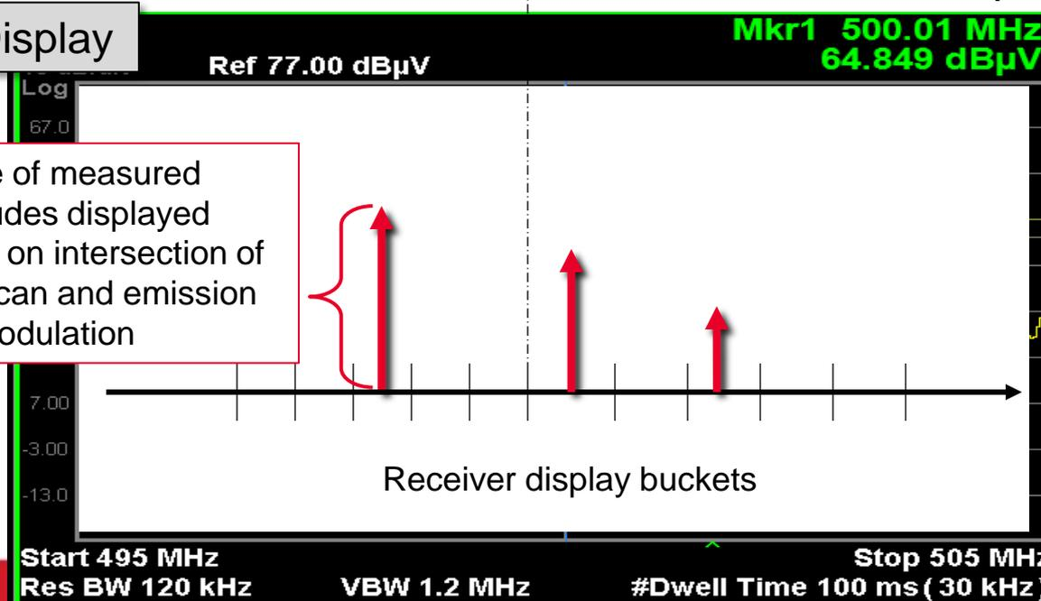
Range of measured amplitudes displayed depending on intersection of receiver scan and emission modulation
