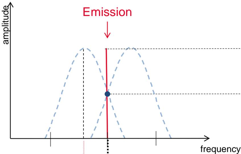
$\Delta f$  ← Max Frequency Error =  $\frac{1}{2}$  step size →  $\Delta f$   $\Delta f$
