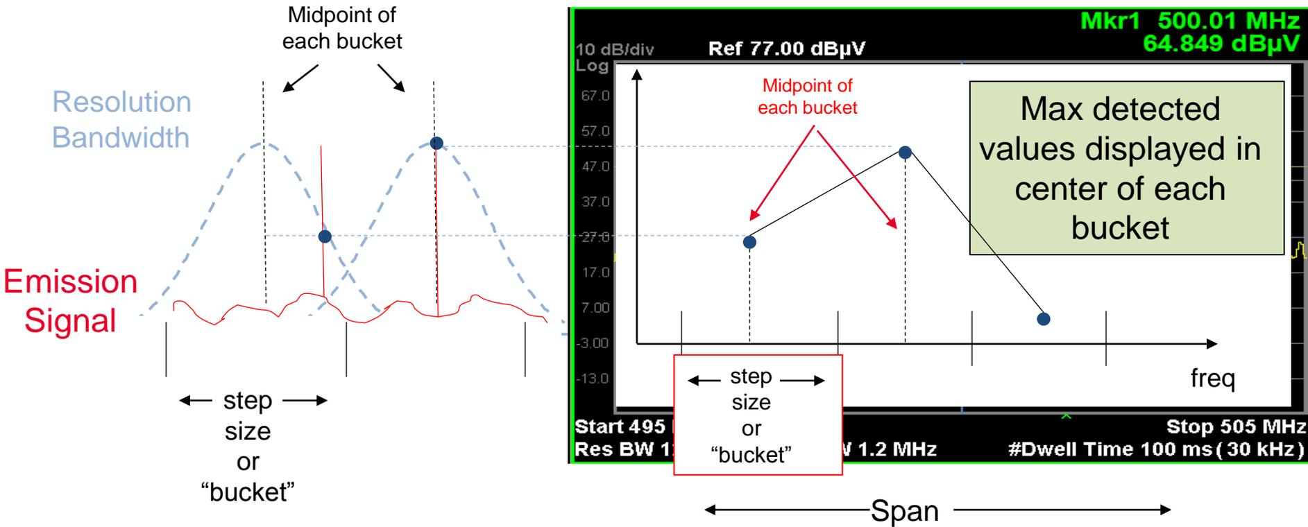
Receivers display amplitudes and frequencies in display “buckets”
