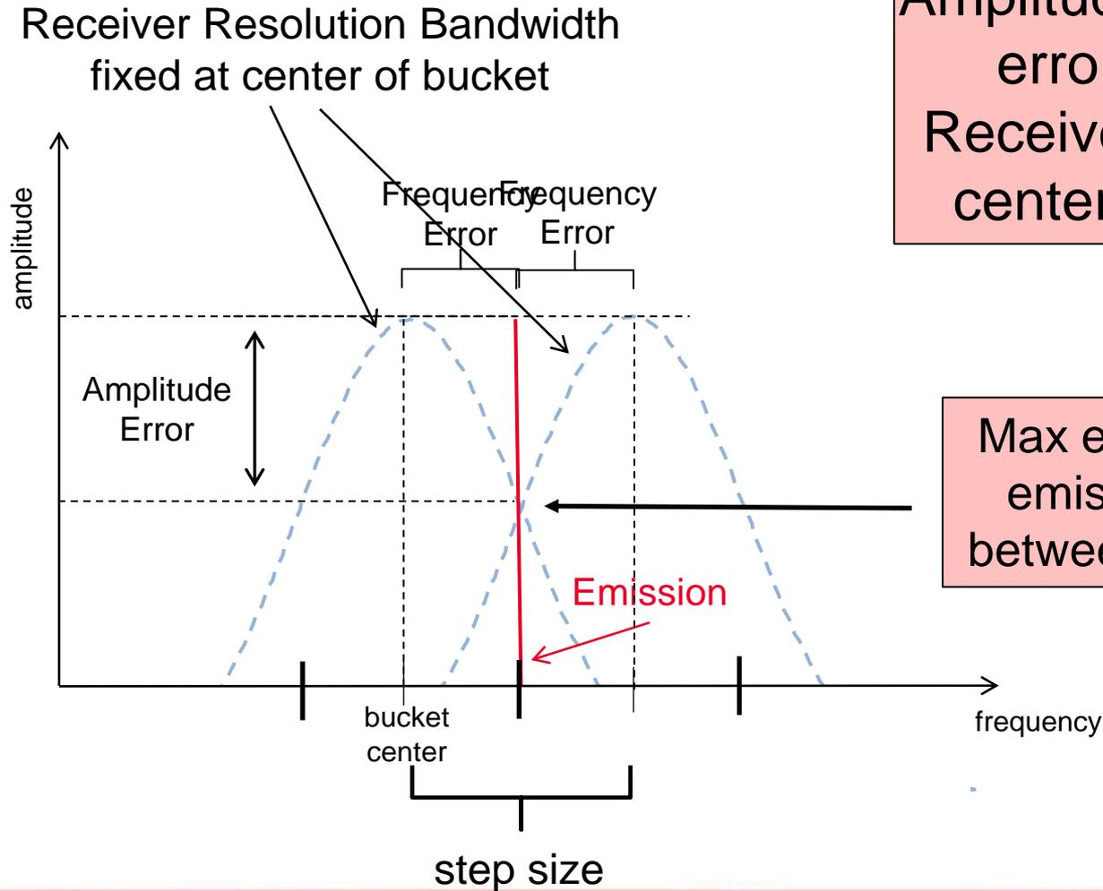
Amplitude and Frequency errors occur when Receiver Bandwidth not centered on emission
