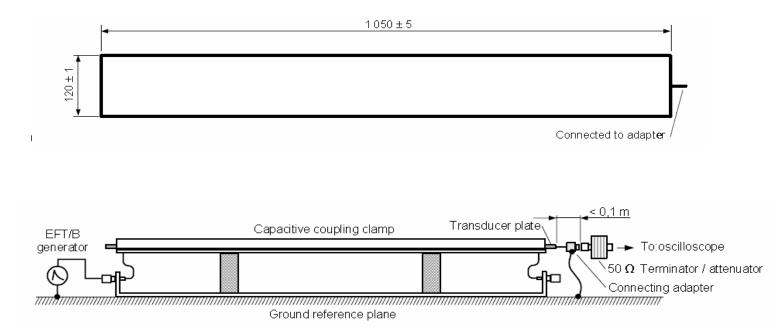
The transducer plate consists in a metallic sheet of 120 mm x 1050 mm of max 0.5 mm thickness, isolated on top and bottom by a dielectric foil of 0.5 mm. Isolation for 5 kV on all sides must be guaranteed in order to avoid the clamp to contact the transducer plate.
