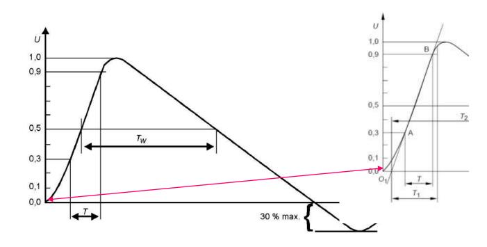
Front time: Duration:  $T_f = 1,67 \times T = 1,2 \ \mu s \pm 30 \ \%$  $T_W = 50 \ \mu s \pm 20 \ \%$ .
