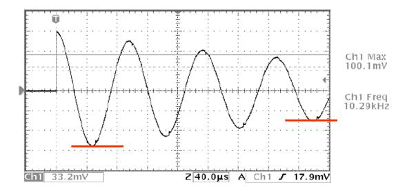
Cosine wave is allowed. In this case Q is calculated from the first full sine wave (NEGATIVE)
