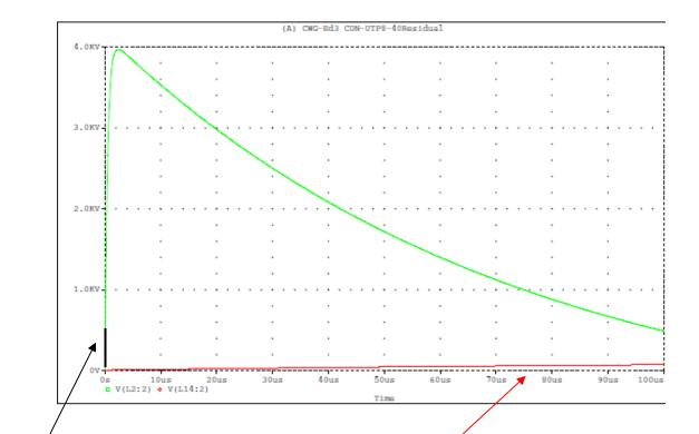
Black curve residual voltage with GDT Red curve residual voltage with linear circuit
