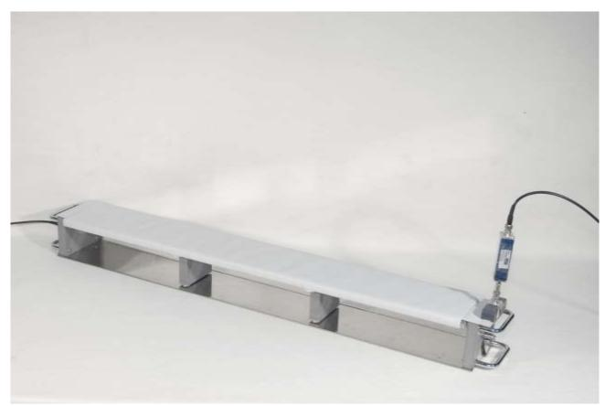
Needs also  $50\Omega$  measurement load impedance
