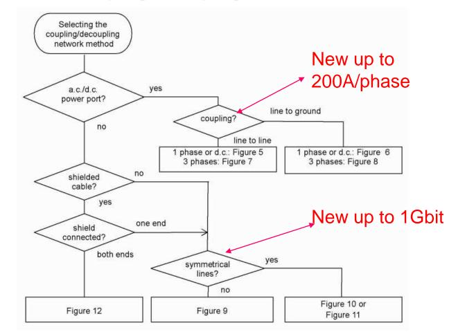
Figure 4: Selection of coupling/decoupling method
