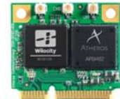
This mini card module for handhelds and other products covers the 2.4, 5, and 60 GHz Wi-Fi bands and includes 2x multiple-input multiple output (MIMO) on the two lower bands for 802.11n compliance. The 60 GHz capability complies with the new FCC 17d standard Bluetooth. A/D also is included.
