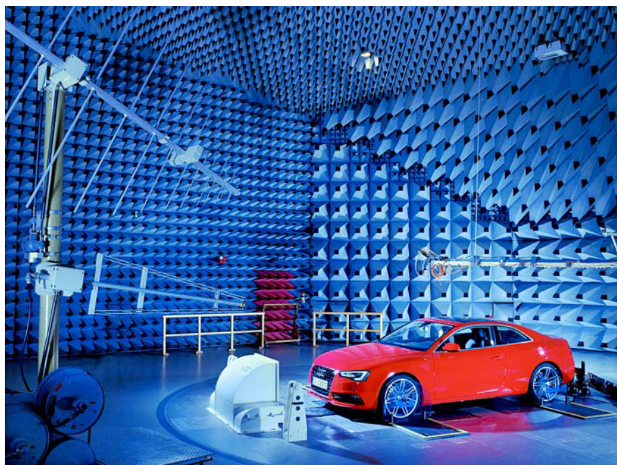
A vehicle being tested to CISPR 12, for interference to objects outside the vehicle.
