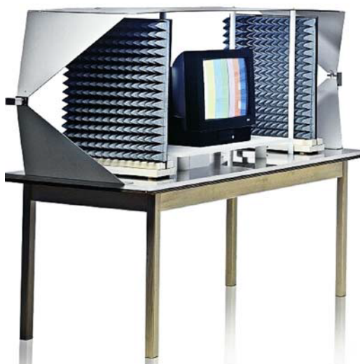
R&S® TS9980 measures the electromagnetic susceptibility (EMS) of sound and TV broadcast receivers, satellite and DVB/DAB receivers in line with EN 55020 and CISPR 20 standards.
