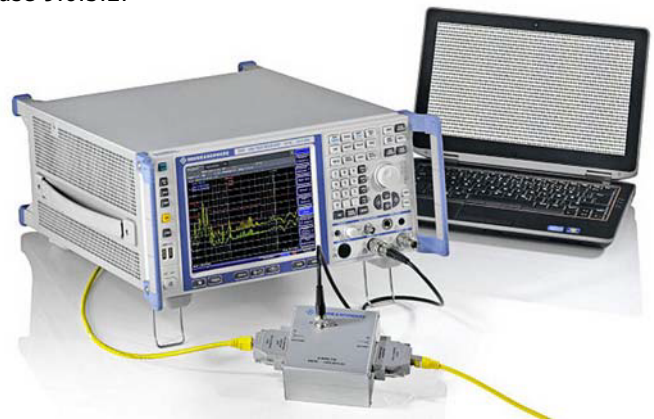
IT equipment such as laptops are subject to CISPR 22 measured here using the R&S®ENY81 and R&S®ESR.
